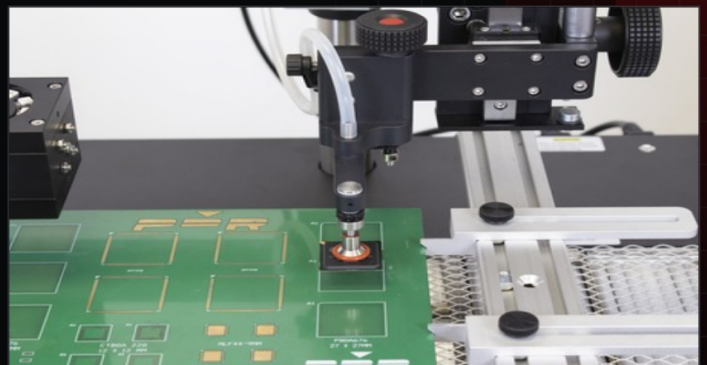
AUTOMATED REMOVAL + PLACEMENT
