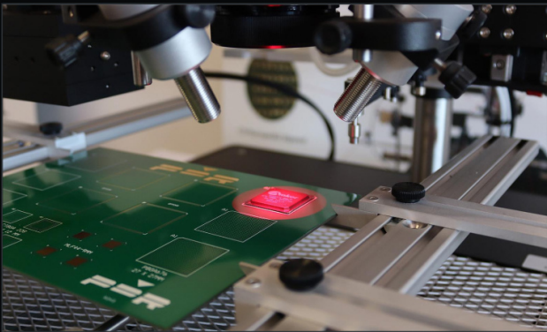
FOCUSED INFRARED | TARGETED COMPONENT HEATING
