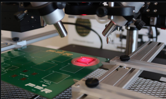
FOCUSED INFRARED | TARGETED COMPONENT HEATING
